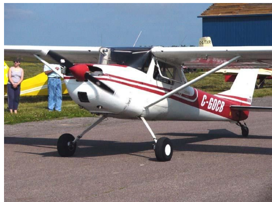
Figure 12: Two front wheels, rear steer [23]
